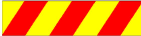
They must be applied to the rear of all vehicles for transporting things that exceed the mass of 3.5 t when fully loaded.
