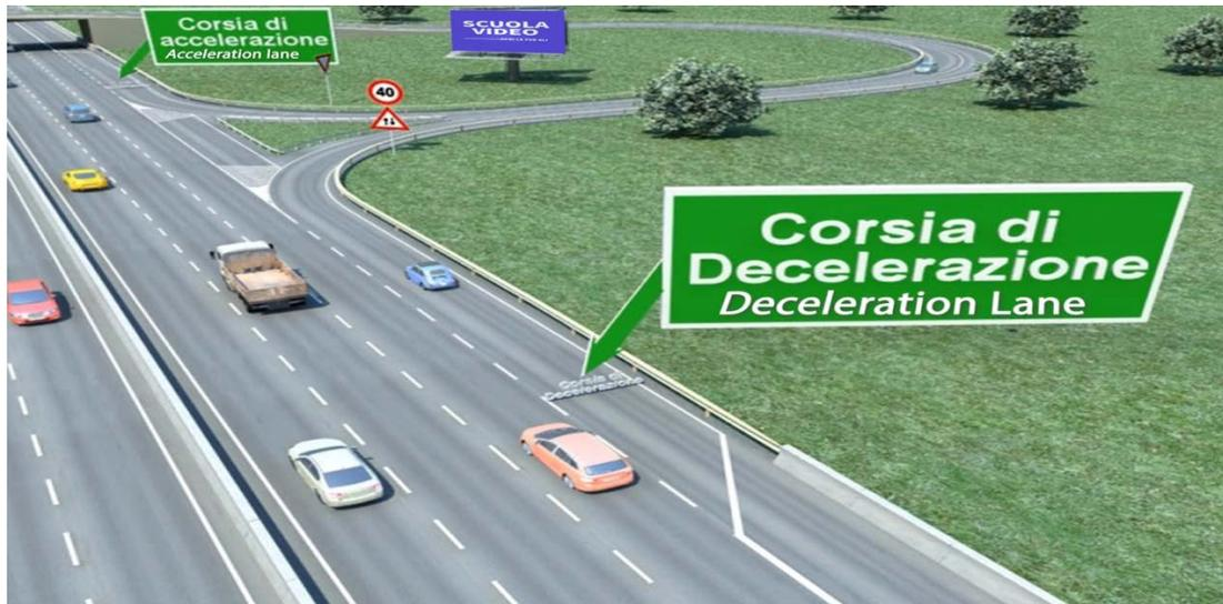
The deceleration lane is used to slow down vehicles when exiting a carriageway or a right-of-way street.
