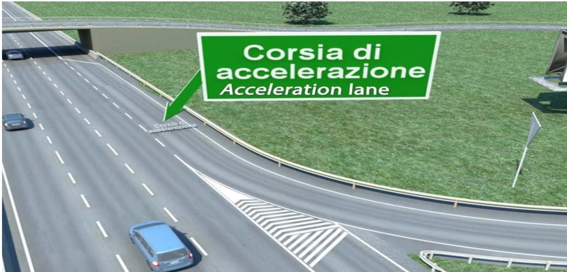
The acceleration lane is used to increase the speed of vehicles entering a carriageway (on a motorway or main suburban roads).
